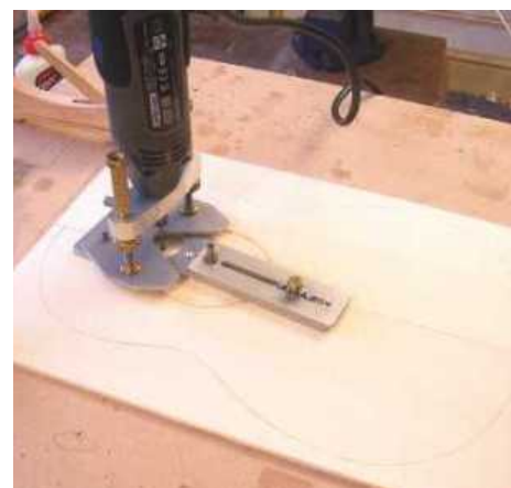
STEP 2. Cutting the rosette channel with the aid of a mini router
